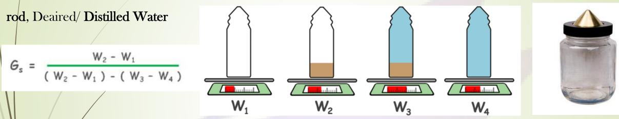
$W_1$  = Weight of the empty, clean and dry pycnometer.
