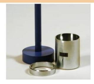
M1 = mass or weight of empty core cutter M2 = mass or weight of core cutter full of soil
