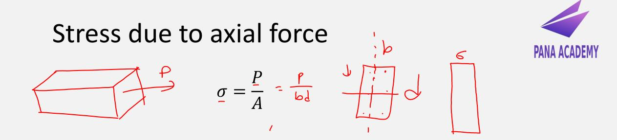
Stress diagram is rectangular with constant stress throughout cross section.
